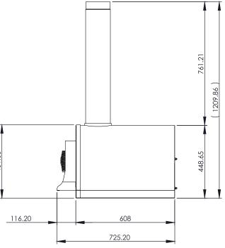
**Overral Dimensions** 725mm Deep x 1007mm Wide x 450mm High x 125kg Weight **Oven Dimensions** 510mm Deep x 790mm Wide x 295mm High
