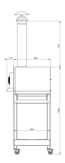
**Overral Dimensions** 725mm Deep x 1007mm Wide x 450mm High x 125kg Weight **Oven Dimensions** 510mm Deep x 790mm Wide x 295mm High
