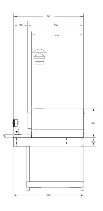
**Overrall Dimensions** 1140mm Deep x 743mm Wide x 502mm High x 125kg Weight **Oven Dimensions** 760mm Deep x 575mm Wide x 355mm High
