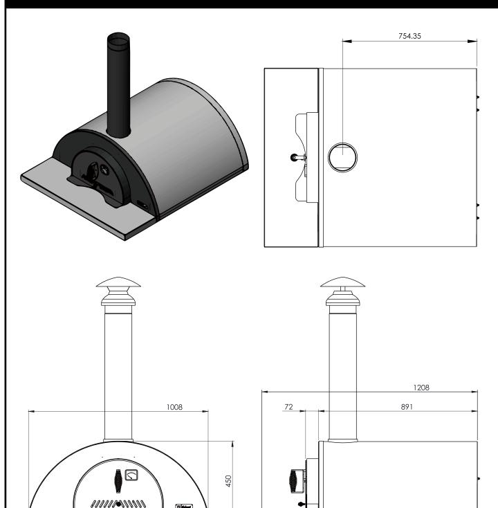
**Overrall Dimensions** 820mm Deep x 900mm Wide x 450mm High x 150kg Weight **Oven Dimensions** 805mm Deep x 805mm Wide x 348mm High
